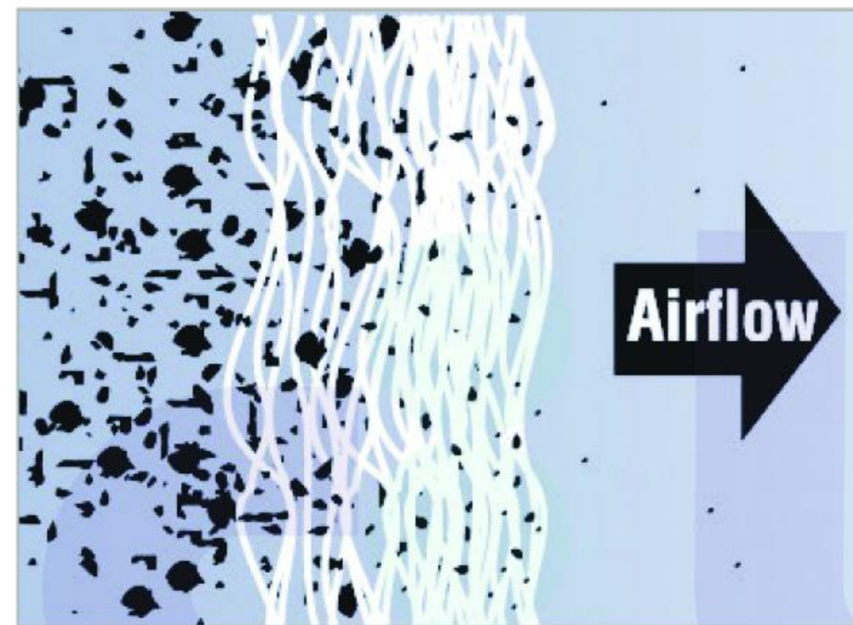
Progressive Density Media Construction
